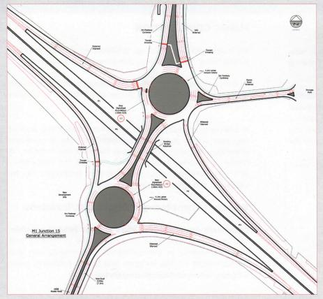
The applicants are exploring ways to improve Junction 15 with a view to helping eliminate peak hour congestion. The plan opposite shows one potential solution currently being considered.
